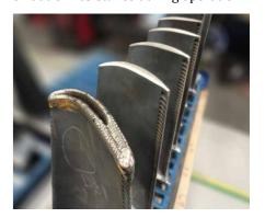
A coating system consisting of a NiCoCrAlY applied by HVOF and a TBC top coat was applied with our propriety coating. The V94.3A4 2nd Stage Blades' lives were extended to operate to a total of 75,000 EOH.
