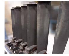
9FA 3rd stage blades were received by our San Antonio facility where they underwent detailed inspections, including microstructural assessment and high-temperature testing.
