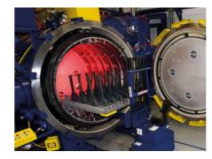
The test blades were evaluated to determine the material's response to the heat treatment. The material responded well to the heat treatment on the blades. The primary gamma transformed to a more cuboidal morphology, which provides for improved component creep life.
